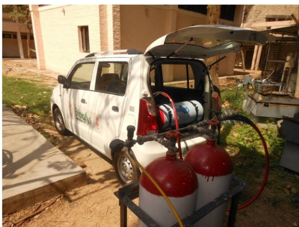
The Bio-CNG dispensing system into vehicles at IIT Delhi.
